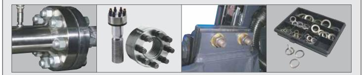
NORD-LOCK washers have cams on one side with a greater rise than the pitch of the bolt. In addition they have radial teeth on the opposite side. The washers are installed in pairs, cam face to cam face. When the bolt and or nut is tightened, the teeth grip and seat the mating surfaces. The tension created makes the bolt / nut self-locking.
